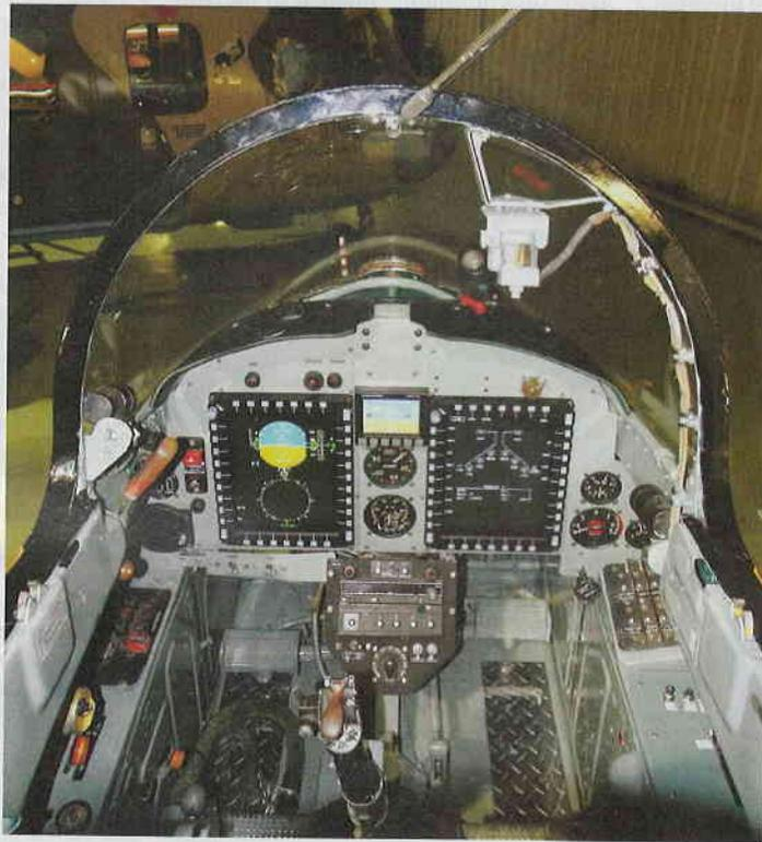
**This L-29 cockpit has been retrofitted with glass to inject real-time virtual adversaries for air-to-air and air-to-ground scenarios.**
